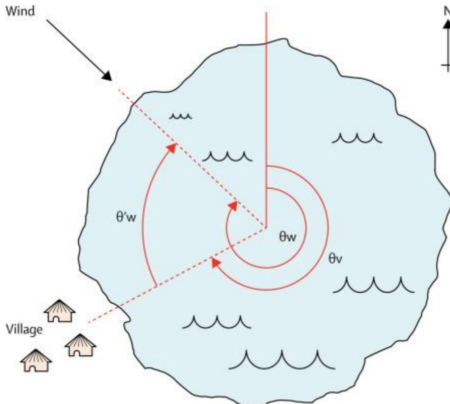
**Figure 2** Definition of wind direction
